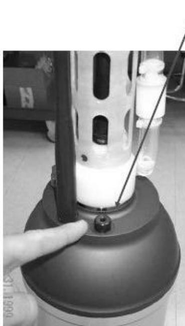
rotate counter –clockwise to unscrew plug.
